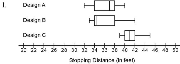
The distance required to stop an Ice Road Trucker and his big rig on a sheet of ice was measured to compare the stopping ability of 3 different tread designs. The results are in the figure below. Which tread design should be chosen if you owned the trucking company?
