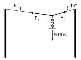
If the traffic signal weighs 50 pounds, what is the tension in the cable that makes the  $16^{\circ}$  angle?
