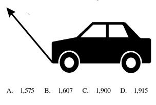
38. A force of 1,000 pounds is required to pull the car up a ramp inclined at  $15^{\circ}$ . To the nearest pound, what is the weight of the car?
